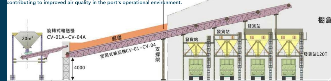
Schematic of the shielded coal discharging facility
