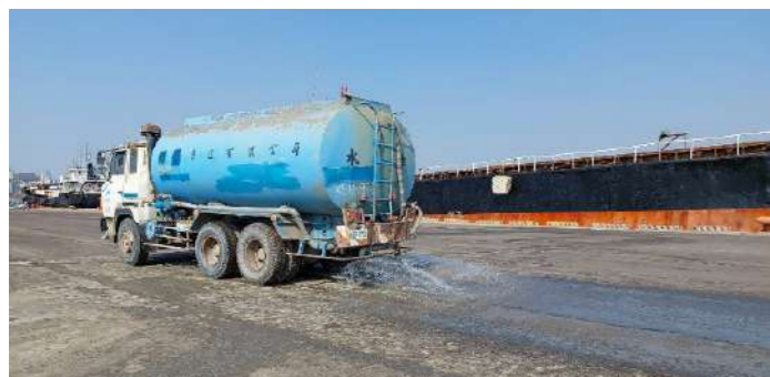
Water Spraying During Loading/Unloading Operations to Reduce Dust
