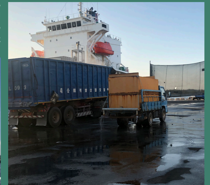
Install dust-proof nets and strengthen watering during loading and unloading operations
