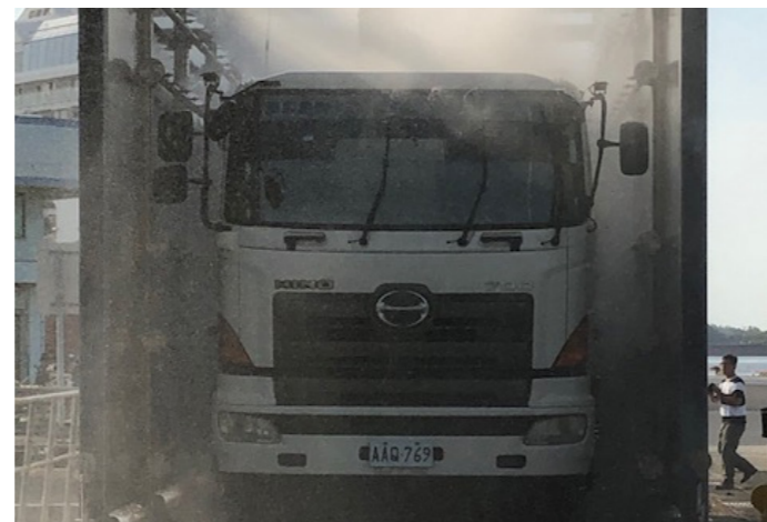
All loading and unloading vehicles must pass through the car wash pool before they can leave
